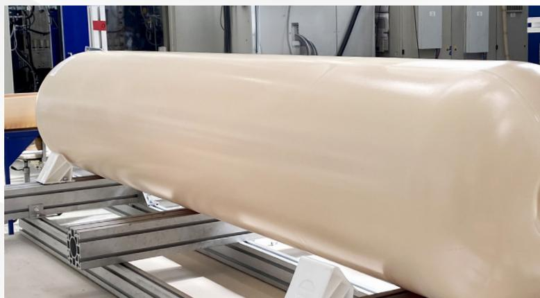
The ability to measure the wall thickness of hot products and make immediate adjustments to the WDS® (Wall-Thickness-Control) has optimized production processes at KAUTEX. The time savings of more than 80% in wall thickness measurement is not only due to the overall speed of the measurement principle but also to the documentation of the measurement results.
