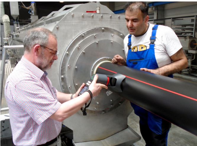
WARP portable in field use with WKT. Stefan Depmer, Head of Technology and Operations, and Türkayan Güneyik, Operations Manager PE, check the pipe wall thickness during the ongoing production process.
