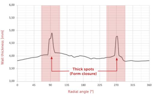
The diagram shows the wall thickness of a liner around the circumference. You can clearly see the thicknesses at the seams of the tool with an otherwise homogeneous wall thickness distribution around the circumference. A scan along the cylinder (cf. barrel measurement) is also possible for the reliable identification of pressure fluctuations in the extruder, for example, which manifest in wall thickness fluctuations.
