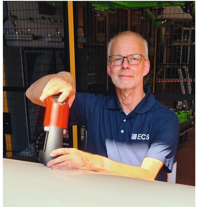
Siegfried Eckert (Managing Director of ECS Service GmbH) measuring a liner with the WARP Portable from iNOEX
